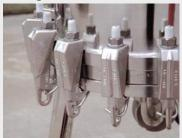
Closing mechanism with swing bolts.
